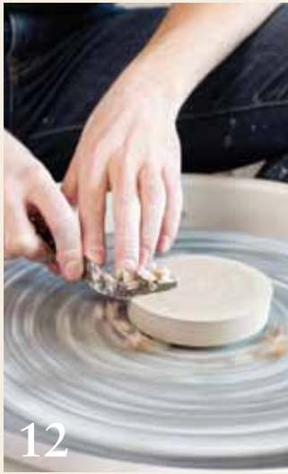
12 Trim excess clay from the top of the lid with a steel turning/trimming tool.
