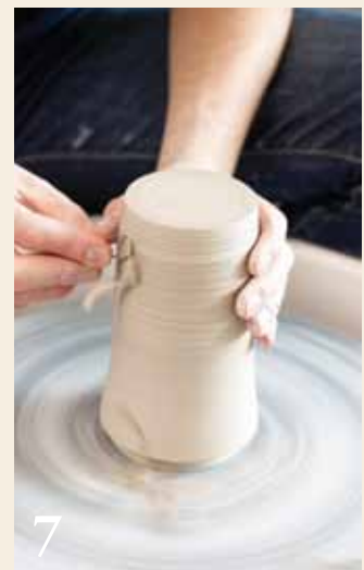
Trim the exterior wall of the leather-hard jar using a ribbon trimming tool.
