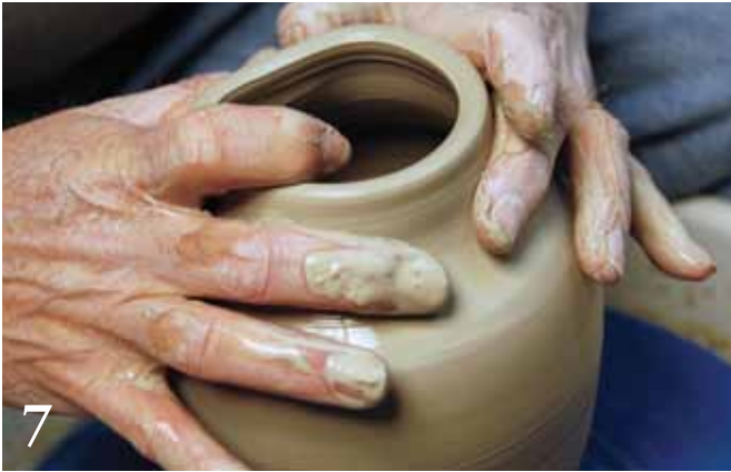
7 Collaring the neck. The middle fingers confine the shape, thumbs push in, first finger of right hand presses down on the rim keeping it level.
