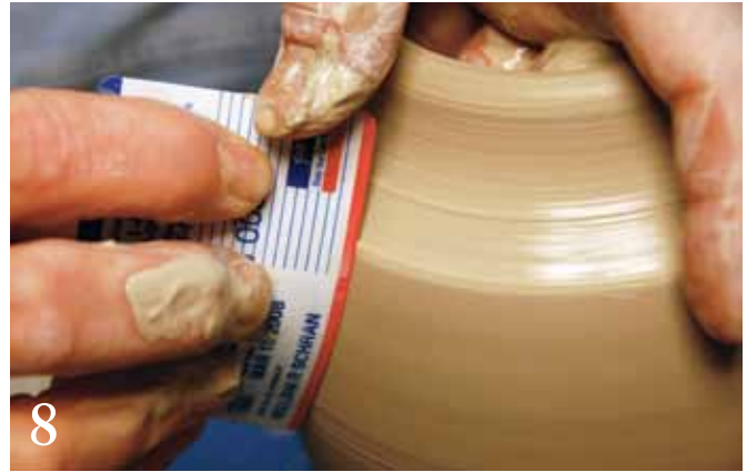
8 A flexible rib removes water and slurry while compressing and refining the wall.
