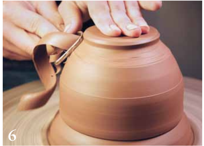
6 Trim away excess clay to define the foot ring.
