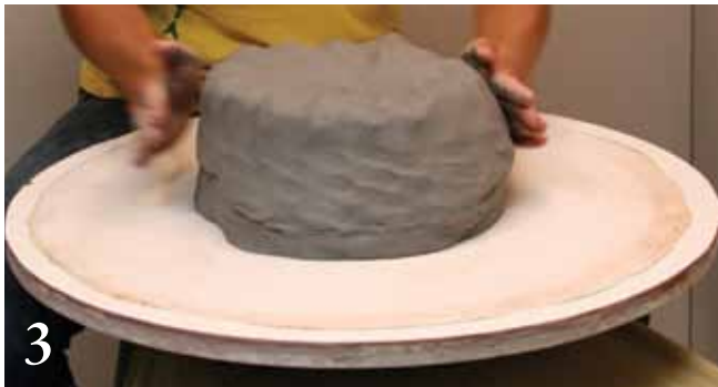
3 Place the ball of clay onto the bat and pound it down into a mound with your hands while the wheel spins.
