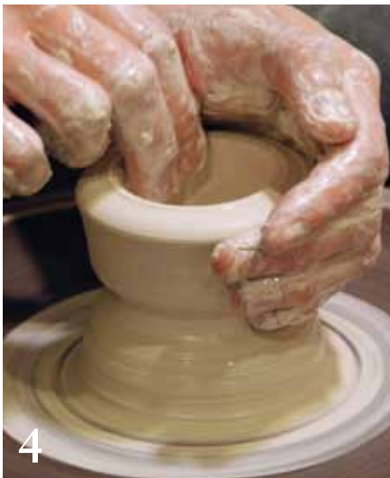
4 Start the spout by throwing a 3–4 inch collared, bottomless cylinder off the hump.
