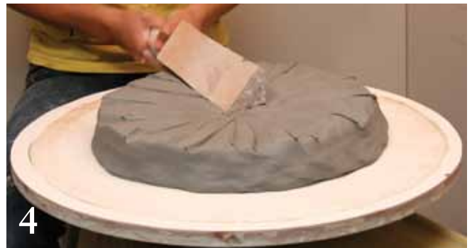
4 As the wheel spins, use a wooden paddle to further compress and flatten the mound until it's between 3–5 inches tall.
