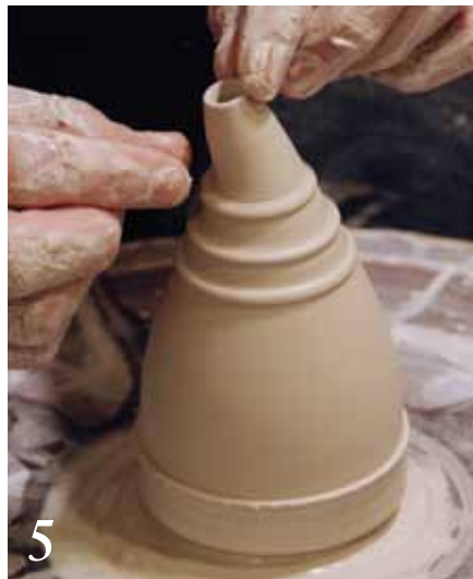
5 Apply decorative rings, and add a kink to the spout by lightly touching the tip.
