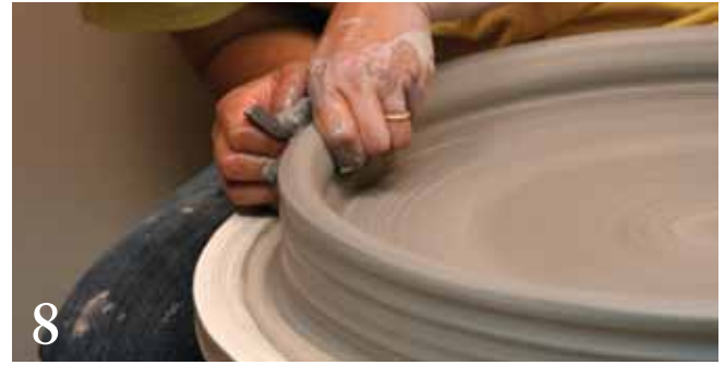
8 Pull the wall straight up using your index finger on the inside and a sponge and the knuckles of your other hand on the outside. Compress the rim after the pull.
