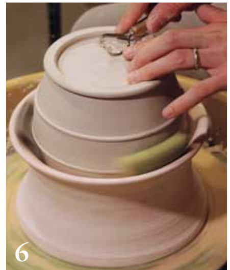
6 Place the teapot body into a chuck with pieces of cut foam to cushion the pot.
