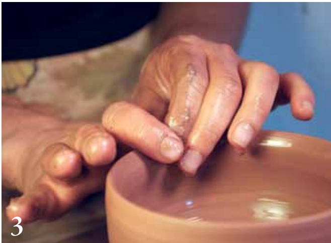
3 Compress the lip using your index finger.
