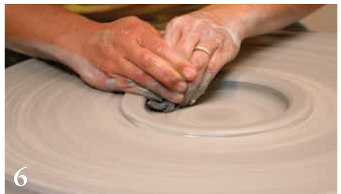
6 Wet your hands and hold a wet sponge in your dominant hand. Press down with both hands to open the form.
