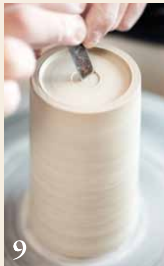
9 Trim a foot ring into the base. Add a trimmed circle for a stamp.
