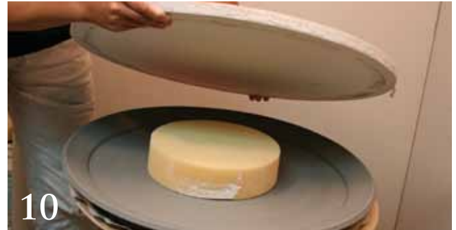
10 Place a foam sheet onto the center of the plate for support while flipping it over.
