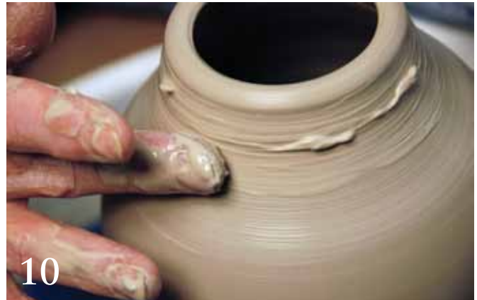
10 Use slurry to lubricate the exterior to maintain a stronger clay wall.
