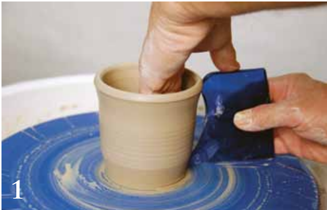
1 Template held against basic cylindrical form.
