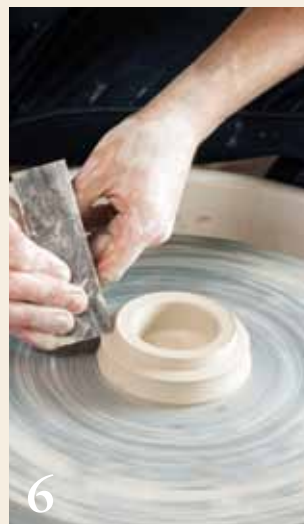
Remove excess clay from the lid and refine the lid's flange with a steel rib.
