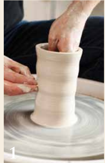
Throwing the jar. An appropriate height is usually achieved in three pulls.
