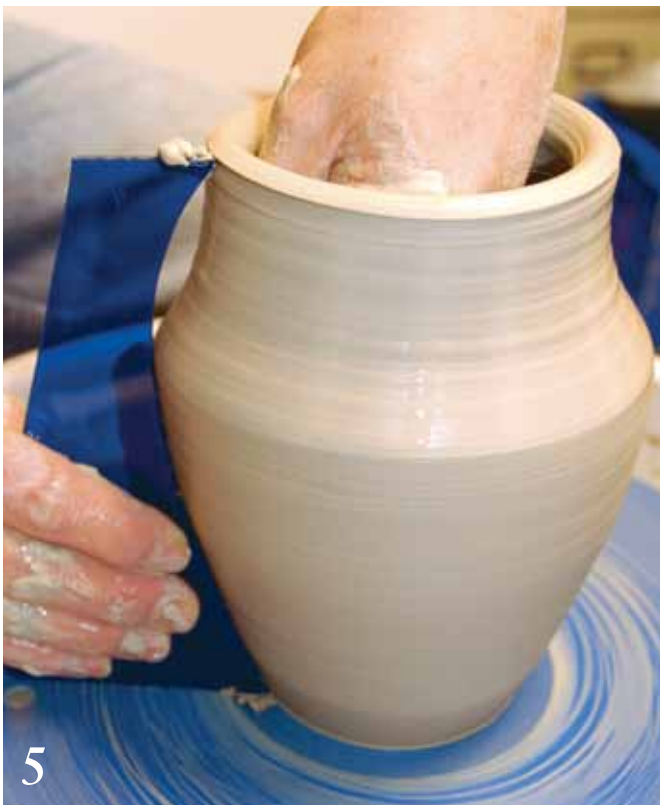
5 The interior hand slowly moves up, pushing the clay against the template.
