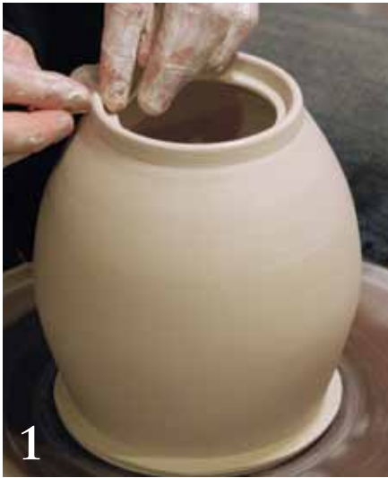
1 Throw and form the body. Leave a thick rim to create the flange for the lid.
