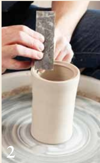
2 Throwing the gallery with a steel rib.
