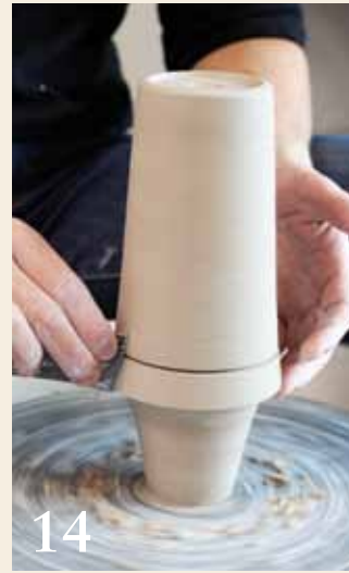
14 Align the lid and jar, trimming the exterior walls using a steel kidney.
