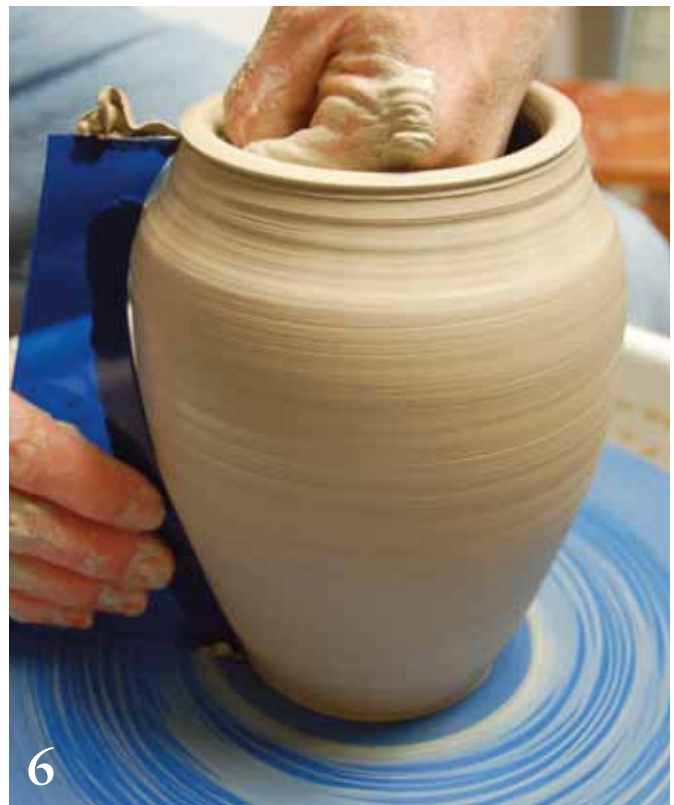
6 The interior hand moves from the top to the bottom, making certain the pot conforms to the template.
