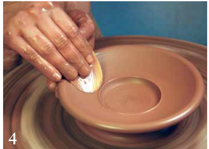
4 Use a stiff rib to define the surface.
