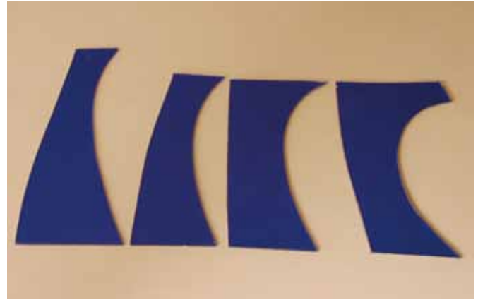
Template shapes used to throw bottle forms.
