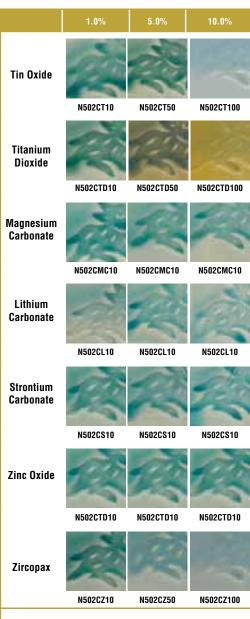
Opacifiers were added to glaze base N502 in increments. The chart above shows which materials were added for this purpose, and the percentages tested. All glazes in this test batch also had 1% copper carbonate added to increase the visual effect of the chemicals on the glaze.
