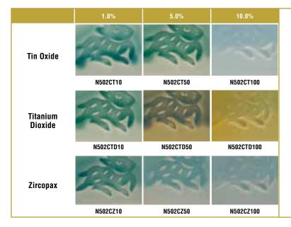
Opacifiers were added to glaze base N502 in increments. The chart at left shows which materials were added for this purpose, and the percentages tested. All glazes in this test batch also had 1% copper carbonate added to increase the visual effect of the chemicals on the glaze.
